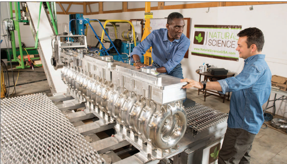
The magnetic system for water applications consists of solenoidal (doughnut shaped) magnets that are coupled together in groups of six to form a module. Several modules are connected together to form an electromagnetic-boom (e-boom) structure. The system can be made longer or shorter by adding or removing modules to accommodate the situation. Every magnet in the structure is separated from the next by a fixed distance that optimizes the ‘gradient’ effect of the magnetic fields between them.
